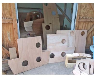
Getting ready to glue down the floor pieces, we spent a Sunday afternoon using a router to cut holes for the various hatches and ports.
